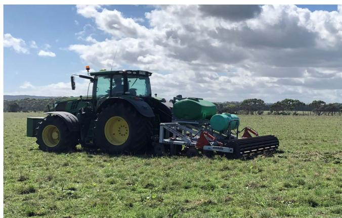
Yeomans Plough with tank for applying treatments
