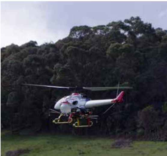
Photo left; the Yamaha R-Max unmanned helicopter demonstrating to the field day attendees targeted blackberry and ragwort spraying
